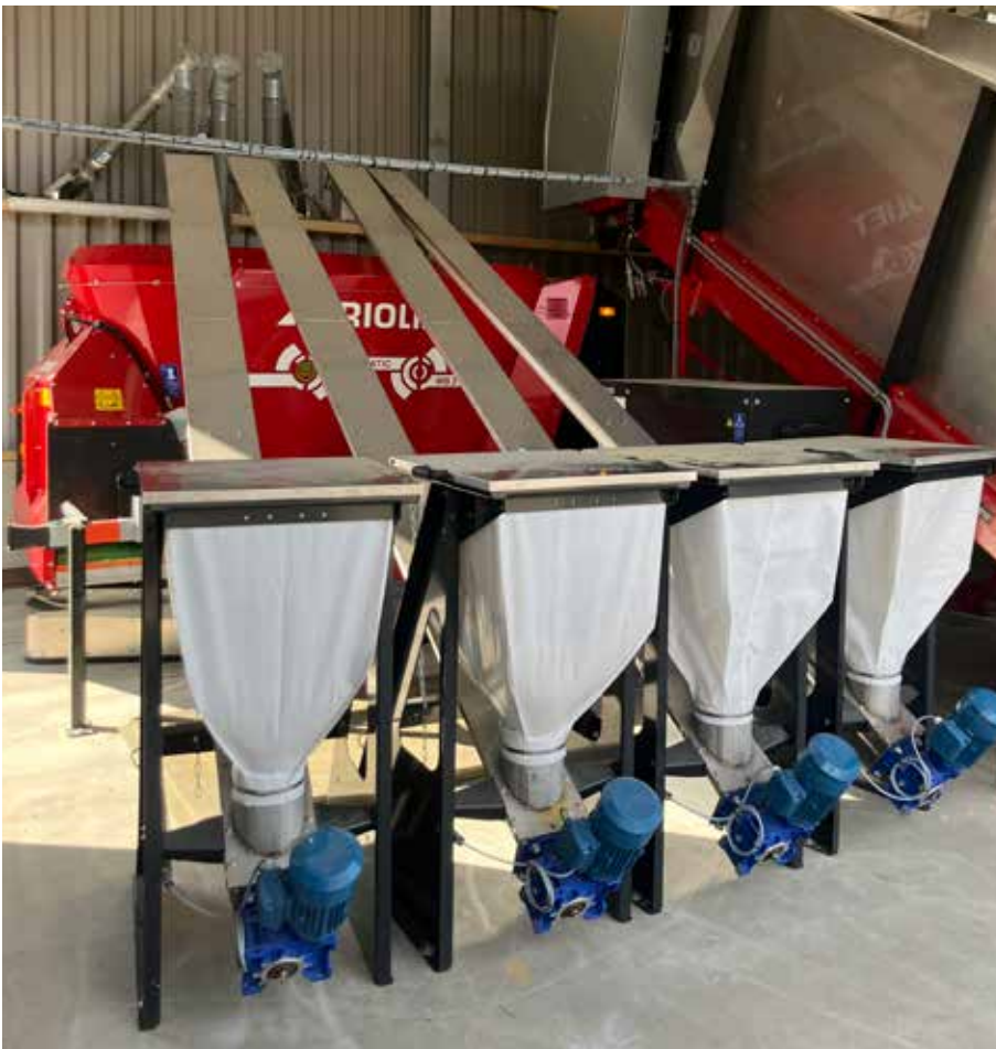
Mineral dispenser with 120 L / 31.7 Gallon storage bag and stainless-steel trough auger
