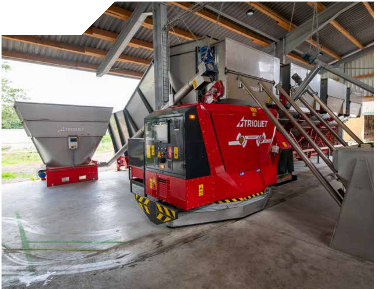
Stainless-steel auger dosing bunker with agitator, cross auger and elevator auger
